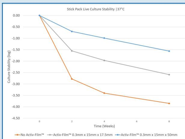
Figure 8: Probiotic Stick Pack Live Culture Stability (CSP Activ-Film™ vs. Standard Foil Packaging without Activ-Film™)
