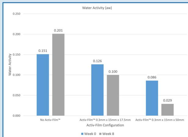
Figure 7: Probiotic Stick Pack Water Activity (CSP Activ-Film™ vs. Standard Foil Packaging without Activ-Film™)
