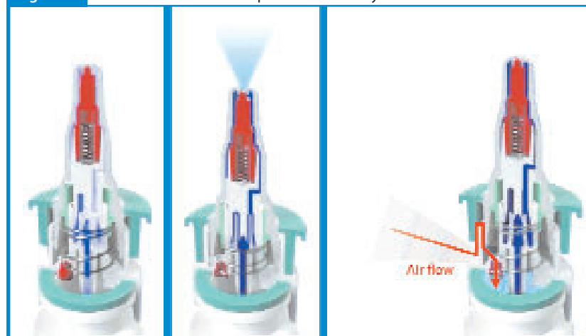
Figure 3: Function of a mechanical preservative-free system.
